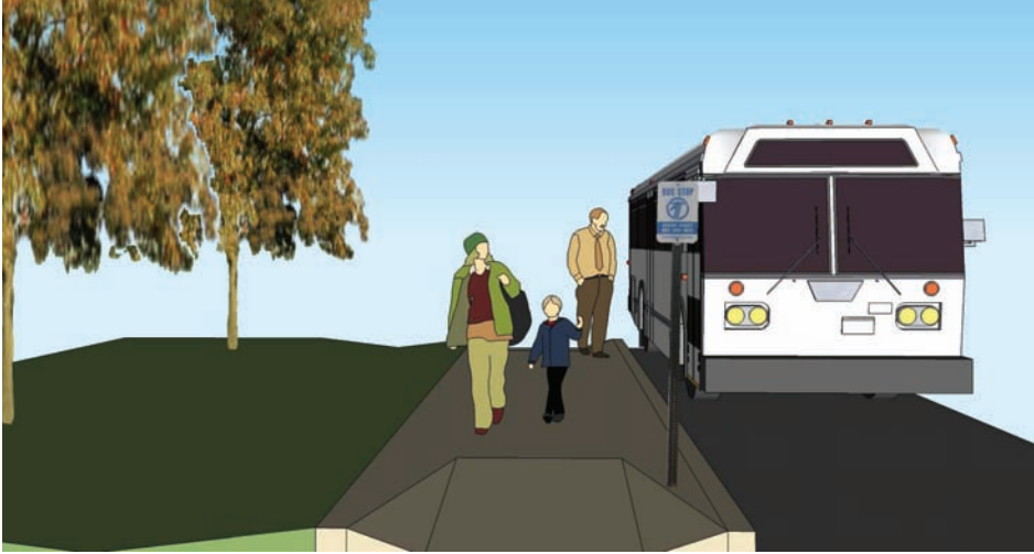
An accessible C Level or rural road bus stop with a landing pad and accessible route. This can connect to a shoulder by curb ramps at either end of the sidewalk.
