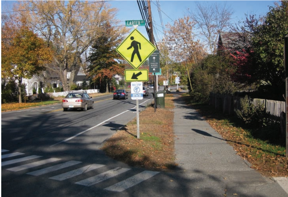
Additional signage at crosswalks is often needed to warn cars of potential pedestrian crossings near bus stops.
