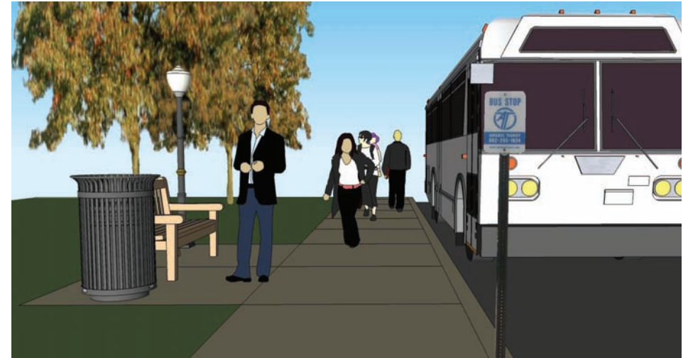
Accessible bus stop without a streetside bufferzone and a landing pad and pedestrian accessible route.
